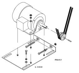
Insert cap screws in tapped removal holes and tighten evenly until bushing becomes loose on shaft. Refer to figure "A" on the previous page.
